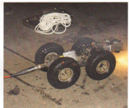
Underground pipe survey module
