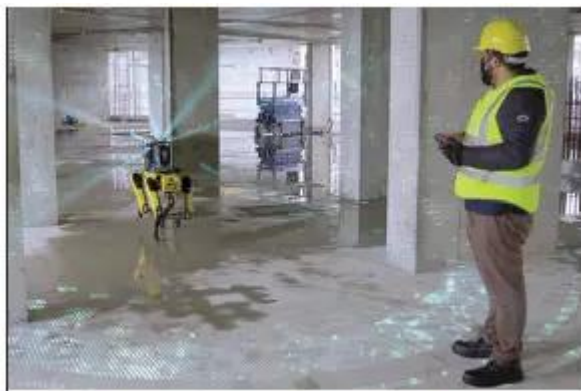
Spot can effectively scan and monitor progress of construction, saving up on time and money.
