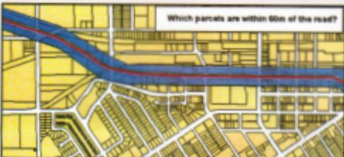
The integration of different data layers involves a process called overlay. At its simplest, this could be a visual operation, but analytical operations require one or more data layers to be joined physically. This overlay, or spatial join, can integrate data on soils, slope, and vegetation, or land ownership with tax assessment.
