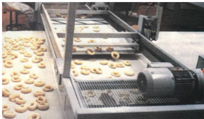
Ammeraal is a Dutch based organisation which specializes in the development and manufacture of process and conveyor belting for light to medium applications. These belts are available in PVC, polyurethane, polyethylene and rubber and have a unique endless jointing system. They are designed for industrial bakeries, food processing plants, airports etc.
